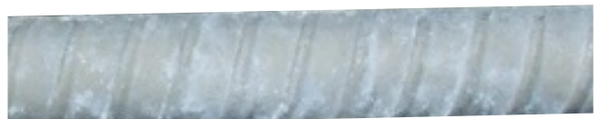
ZINC FLAKE AFTER 1000 HOURS OF SALT SPRAY TESTING
